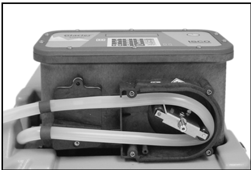
Figure 5-2 Pump housing cover removed
